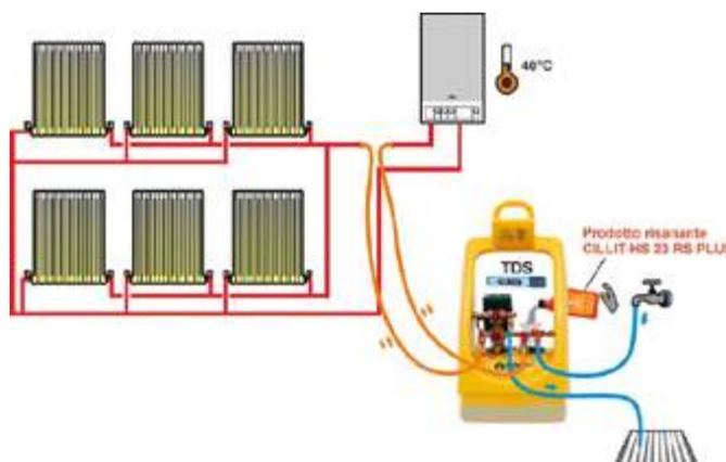
**SCHEMA DI LAVAGGIO CON POMPA SOLUTECH**
