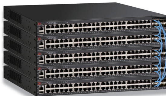
Figure 1: Up to 12 Brocade ICX 7250 Switches can be stacked together using up to four full-duplex SFP+ 10 Gbps ports for a fully redundant backplane with 480 Gbps of aggregated stacking bandwidth.
