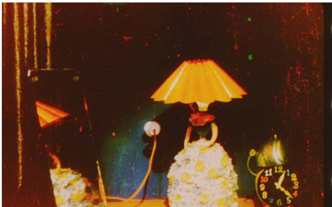
Fig.6. Dirt marks on Gasparcolor seen in colour when the three layers are combined.
