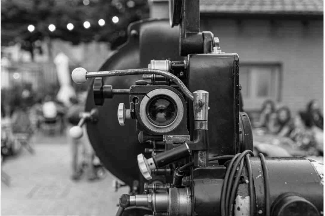
Carbon arc projector used during the festival Il Cinema Ritrovato in Bologna.
