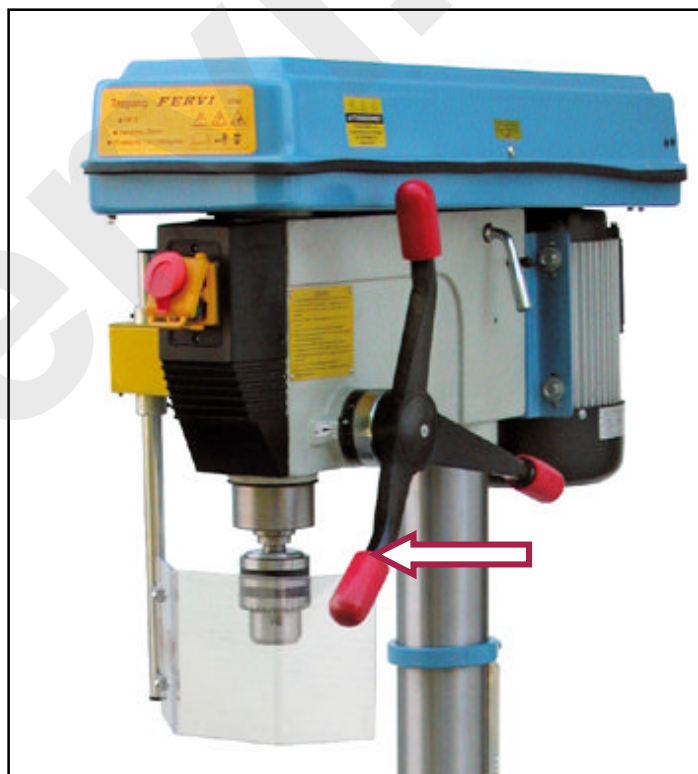
Figure 15 - Hand-wheel for vertical displacement.
