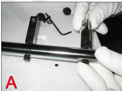
Figure 7 – Application of the brackets (A) – Insert the guard (B).
