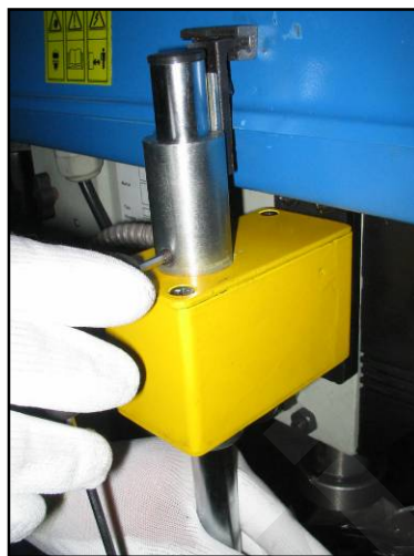
Figure 8 – Installation of the Rod Carrying the Guard.
