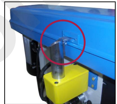
Figure 18 - Pulley compartment locking device.
