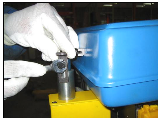
Figure 9 – Fitting and Adjusting the End of the Rod.
