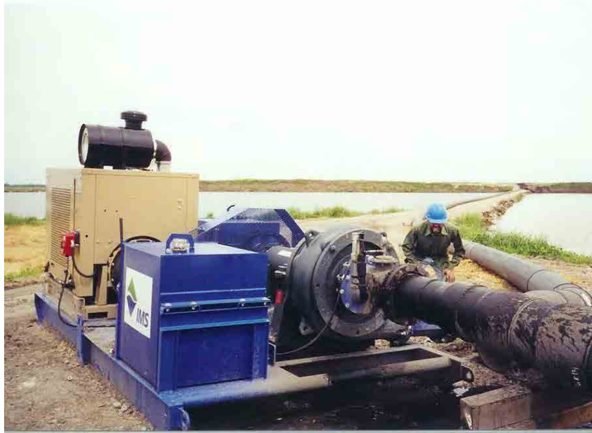
Dredging Booster Pump (Skid Mounted for Inshore Installation)
