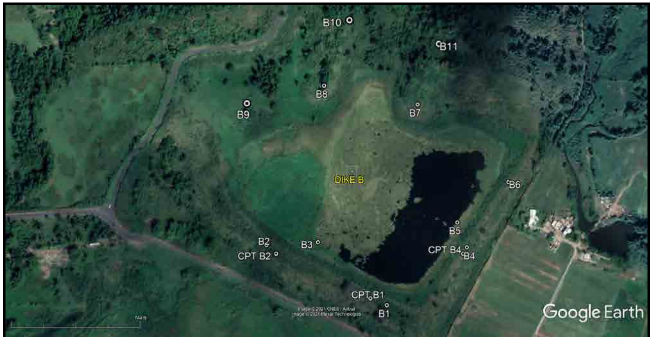
Figure 5. Borings and CPT locations at Dike B.
