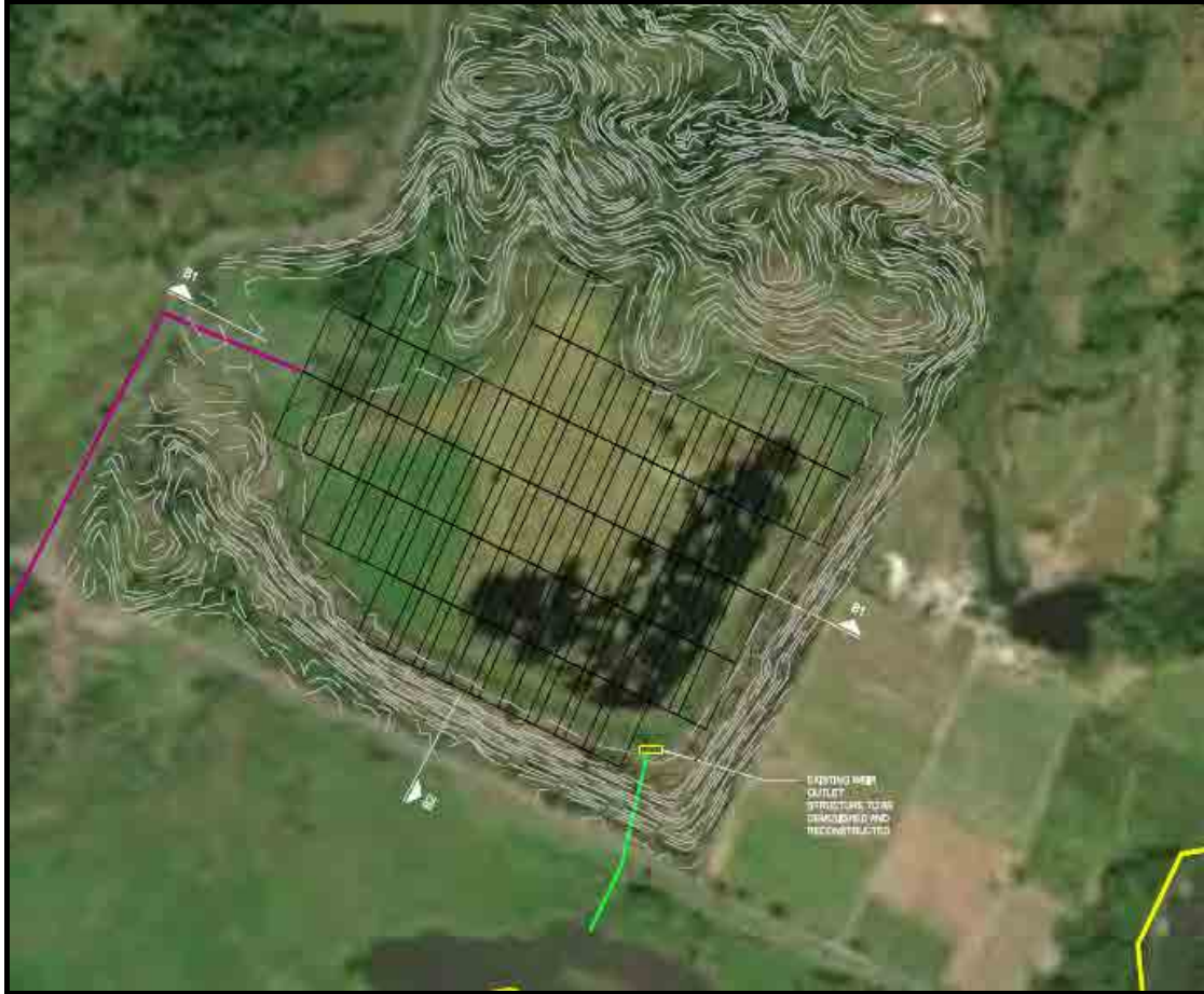
Figure 3. Preliminary array of geotubes inside Dike B (provided by GLM).
