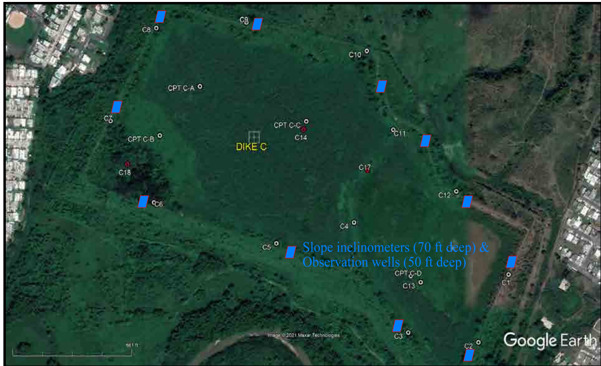
Figure 10. Slope inclinometers required during and after dredge deposition.
