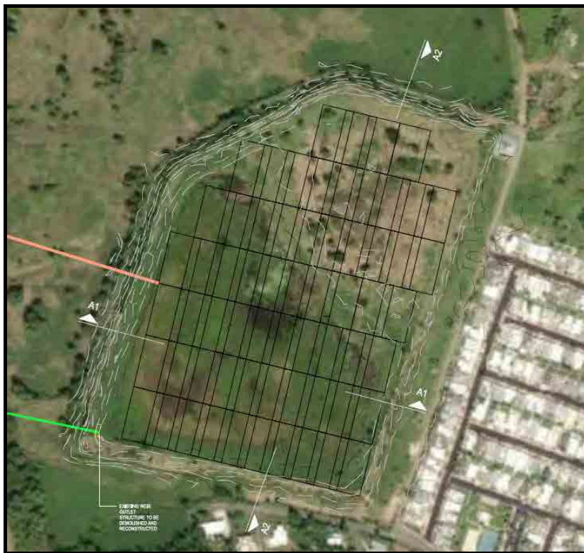
Figure 3. Preliminary array of geotubes inside Dike A (provided by GLM).
