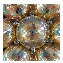
Fig. 25. Photograph showing a real size mock-up of the 3-inch photomultipliers interlaced between the 20-inch ones.
