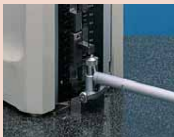
Bore gage zero-setting
