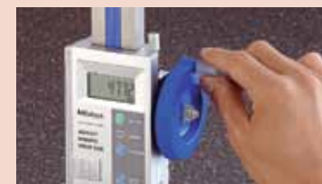
Large smooth slider feed wheel
