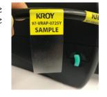
Step 2: Wrap "tail of wire wrap around the wire/cable and over printed area
