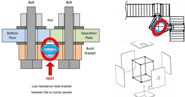
Figure 3: Cleat junction releasing in temperature [17] Figure 4: Structural Bar cut in temperature
