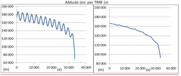
Figure 14: DEBRISK jobs for early re-entry trajectory
