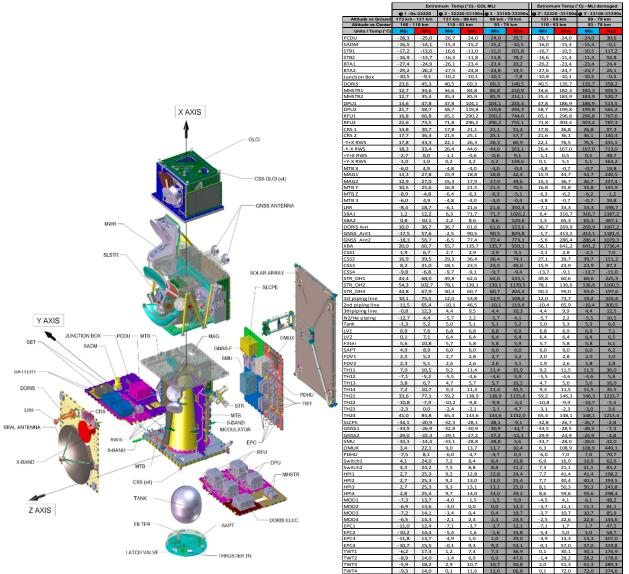
Figure 19: Thermal nodes designation and location on Sentinel-3 exploded view
