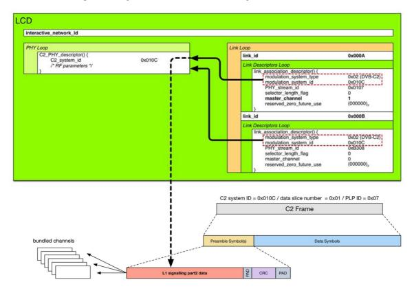
Figure A.6: Example of DVB-C2 channel bundling
