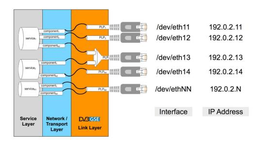
Figure 3: Application programming model of DVB-GSE with LLC
