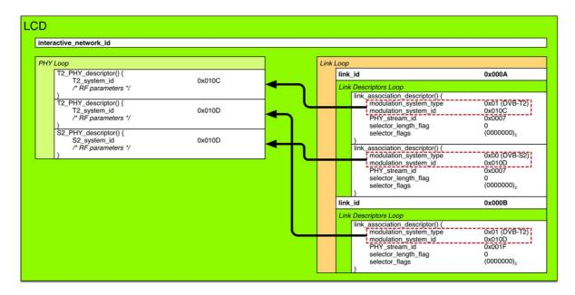
Figure A.5: Example of carriage of Links on different physical layers
