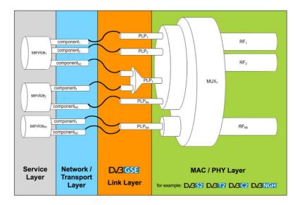
Figure 2: Protocol layers when using DVB-GSE
