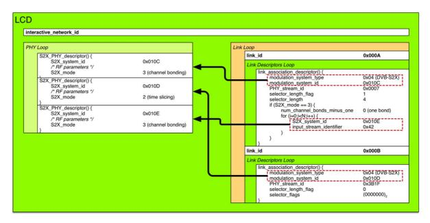
Figure A.7: Example of DVB-S2X channel bonding and time slicing
