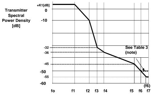
NOTE: Frequency from actual transmitter centre frequency [MHz].
