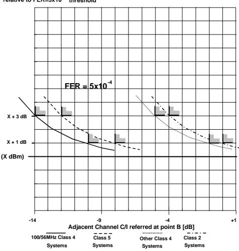
Receiver Input Level at Reference Point C relative to FER=5x10<sup>-4</sup> threshold
