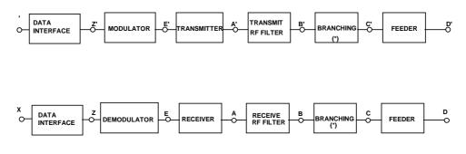
NOTE 1: For the purpose of defining the measurement points, the branching network does not include a hybrid. NOTE 2: The points shown above are reference points only; points C and C', D and D' in general coincide.
