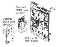
provide connection for powering conventional two-wire smoke detector circuits on Signature Series modules.
