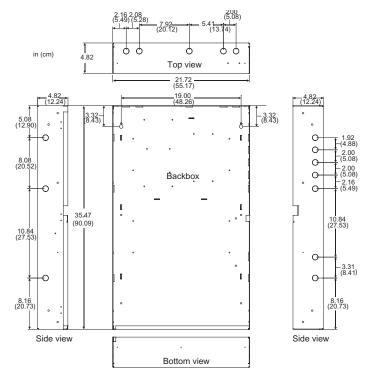
**Note:** Add 0.25 in (0.64 cm). to height and width dimensions to allow for knockouts when framing in the backbox for semiflush mounting.
