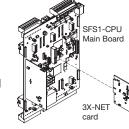
The 3X-NET adapter card provides two independent RS 485 circuits: one for network data communications and one for digital audio communications.
