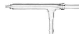
500-72 - C-Type Concentric Nebulizer, 1 lpm Ar, 30psi, 3mL/min
