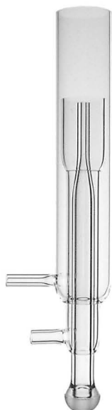
550-20 - 1 Piece Torch with Ball Joint, Aqueous, 120-3748
