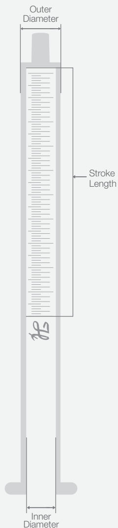
Syringes Figure 7. Syringe dimensions
