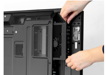
OPS inserted into NEC Large Format Display
