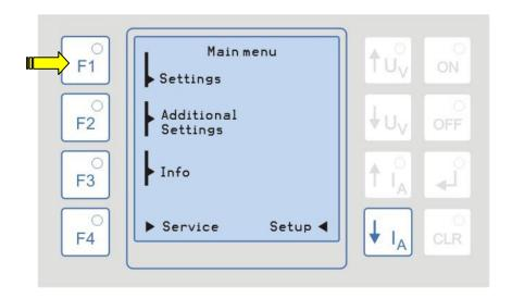
Select the desired menu point by pressing the corresponding key.
