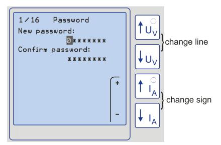
For each digit, select the cipher 0 to 9 by using the keys
