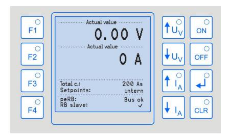
In normal operating mode, the digital display shows the actual current and voltage parameters of the connected DC power supply.
