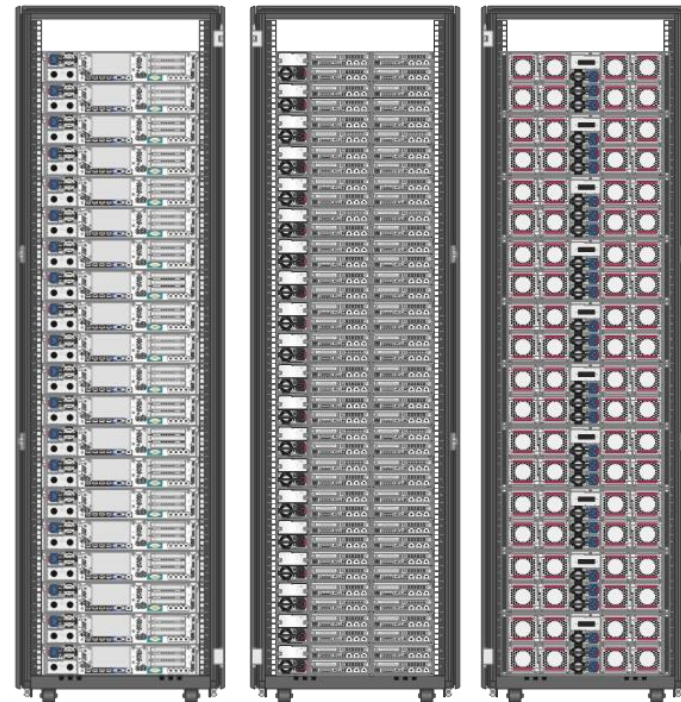
DL380P SL2500 SL6500 20 Servers 40 Servers 80 Servers
