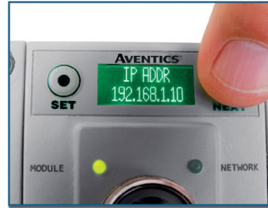
Graphic Display for Configuration & Diagnostics
