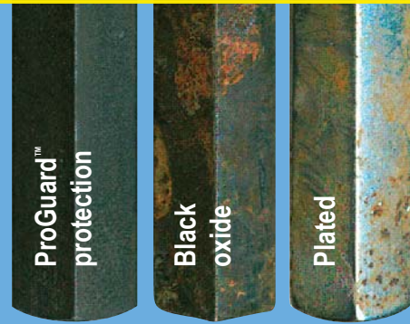
Actual corrosion after 10 hours exposure to salt spray
