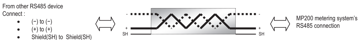
Figure 5.3: 2-wire RS485 Connection
