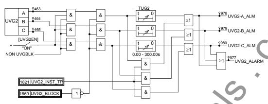
Figure 2.4.9.10 UVG2 Undervoltage Protection
