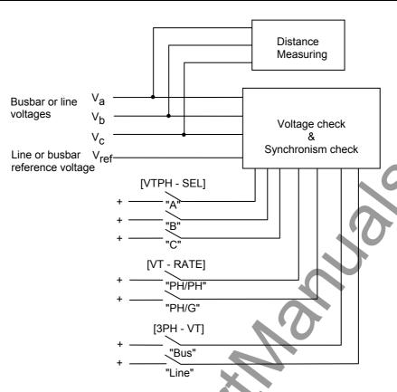
Figure 2.7.2.4 Matching of Busbar Voltage and Line Voltage
