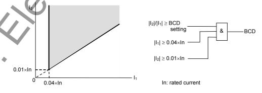
Figure 2.4.10.2 BCD Element Characteristic
