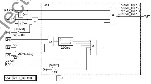
Figure 2.4.3.6 Weak Infeed Trip Logic
