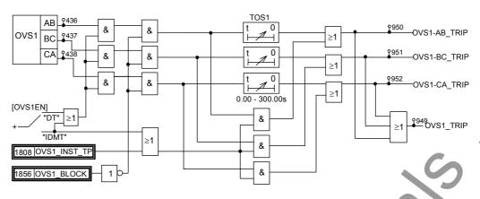
Figure 2.4.9.2 OVS1 Overvoltage Protection
