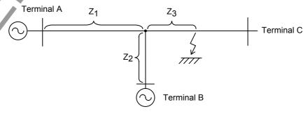
Figure 2.3.2.1 Three-terminal line
