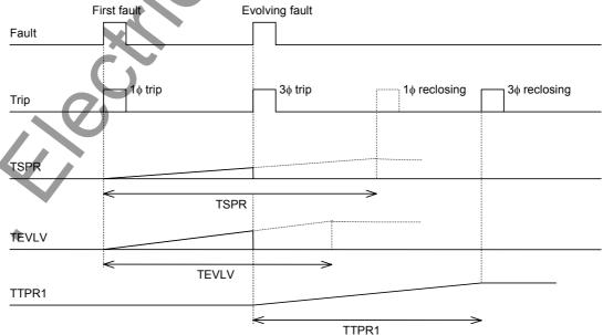
Figure 2.7.2.2 Autoreclose for Evolving Fault
