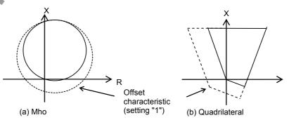
Figure 4.2.7.1 Z1 Characteristics by [ZB-CTRL] Setting
