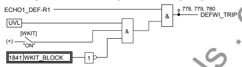
Figure 2.4.4.5 Weak Infeed Trip Logic
