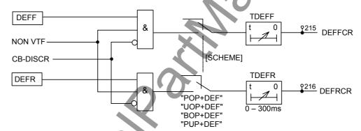
Figure 2.4.4.2 DEF Command Protection
