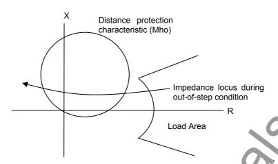
Figure 2.1.5.2 Impedance Locus during Out-of-Step Condition
