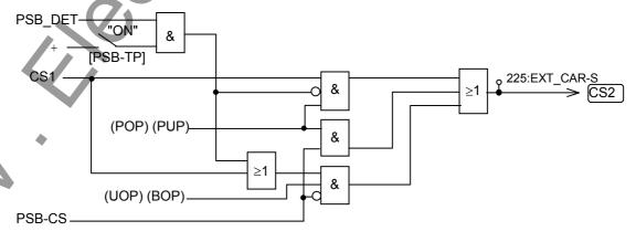
Figure 2.4.15.3 Sending Signal Control in External Communication
