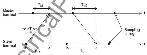
Figure 2.5.1.2 Timing Synchronization
