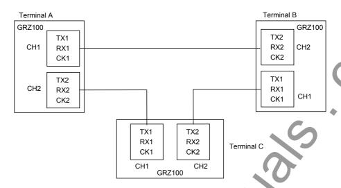
Figure 2.5.1.7 Communication Circuit Setup for Three-terminal Applications
