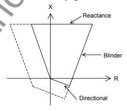
Figure 2.6.1.11 Quadrilateral characteristic
