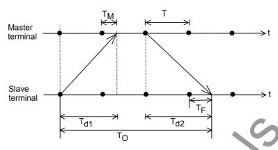
Figure 2.5.1.4 Sampling Address Synchronization
