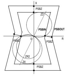
Figure 2.4.15.1 Power Swing Blocking Element
