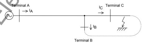
Figure 2.3.2.3 Outfeed Current in Event of External Fault
