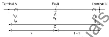
Figure 2.8.4.1 Two-terminal Model
