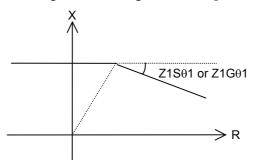
Figure 4.2.7.2 Gradient Characteristic of Zone 1 and Zone 1X
