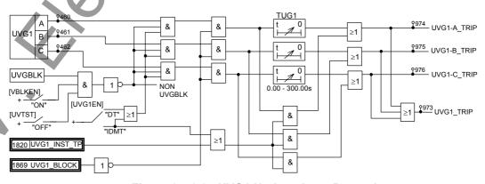
Figure 2.4.9.9 UVG1 Undervoltage Protection
