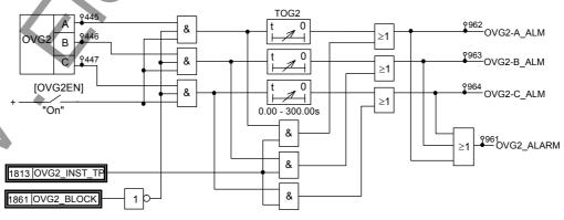
Figure 2.4.9.5 OVG2 Overvoltage Protection
