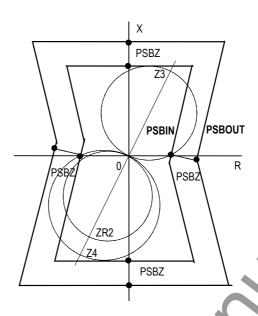
Figure 2.6.1.4 Power Swing Blocking Element
