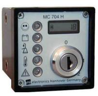
Activating the system is accomplished by turning the key to the start position. After 7seconds from initial start the MC 704 will begin to monitor the inputs. This shutdown delay eliminates the need for pushing an override button commonly required on old fashioned units during start-up.
