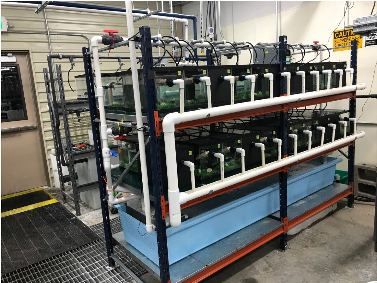
Figure 1. New 44 tank experimental rack built at the UNFH refugia.
