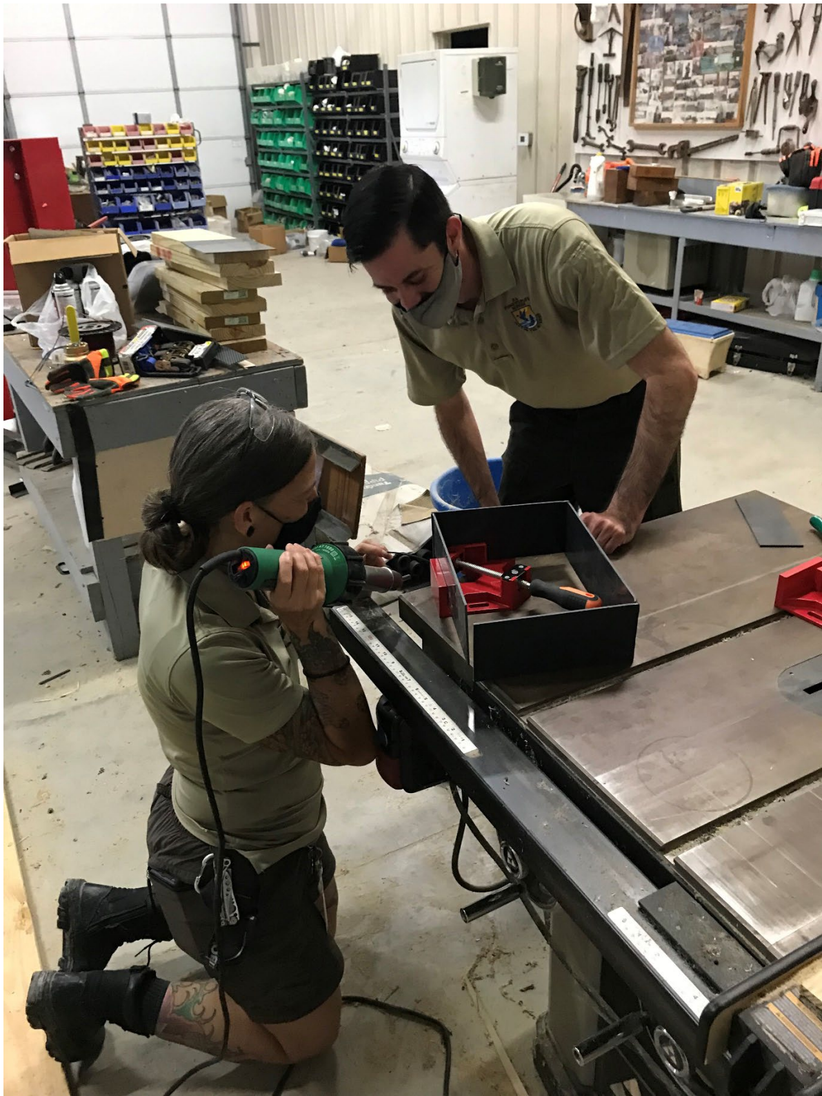
Figure 3. Jennifer Whitt heat welding the corner seams on the filter box that was added to the redesigned invertebrate rack with Adam Daw's supervision.
