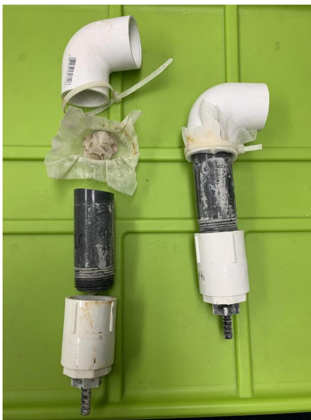
Figure 2. Structure and size of an upwelling flow-through chamber that maintained an air-water interface used in the air space access experiments. Note the pieces of 100 mm Nitex mesh used at the ends to prevent escape or loss of CSRBs and to create an air-water interface.
