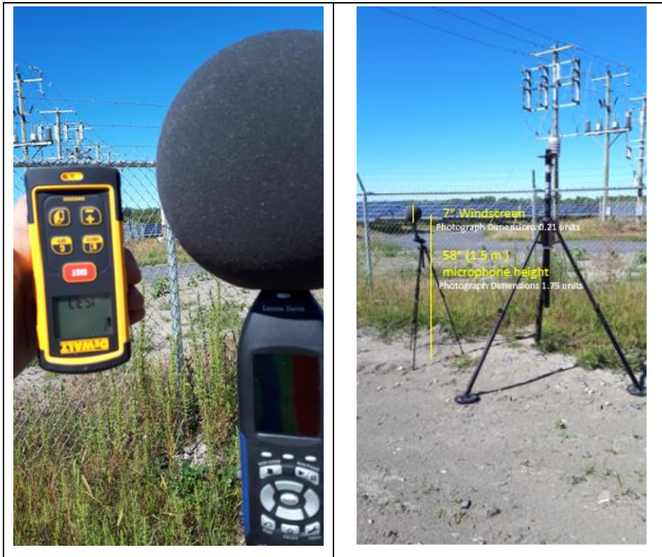
Figure 1-1 Photos of laser distance measurer and relative sizing from the South location
