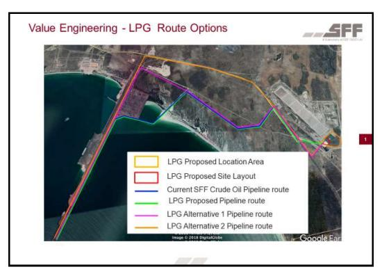
**Figure 1:** Map showing the three alternative pipeline routes assessed, plus the facility location.
