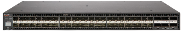
Figure 1: The Ruckus ICX 7750-48F features 48 1/10 GbE SFP+ ports and 6 40 GbE QSFP+ ports that can each be split* into 4x10 GbE SFP+ ports. The front panel also displays the unit stacking ID.
