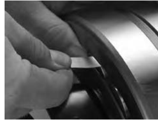
Fig. 3. Measure RIC before installation.
