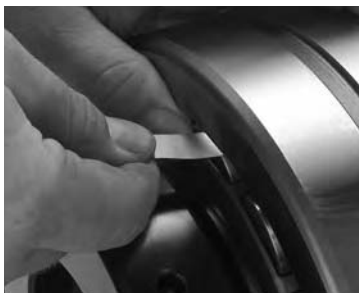
Fig. 7. Measure RIC before installation.
