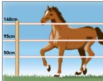
Electric fences for large horses are 1.30 to 1.60 m high with 2 to 3 conducting wires.
