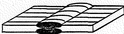
Correct Weld Correct Grind
