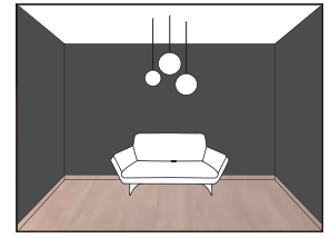
A light floor and ceiling with dark walls make a space seem narrower, deeper and taller.
