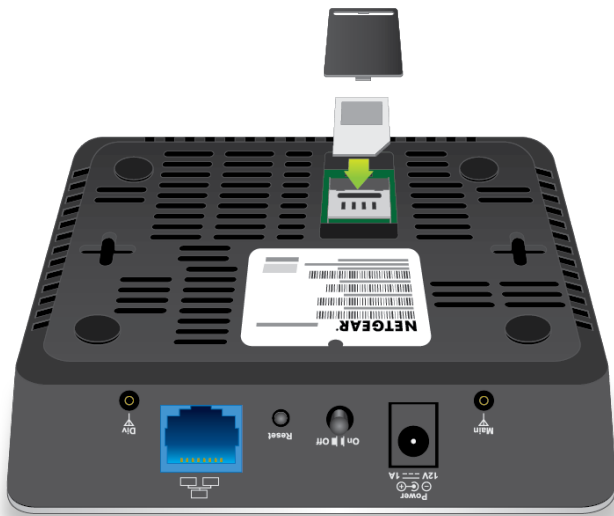
Figure 2. Overview of installing the micro SIM card
