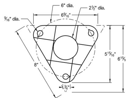
Bolt Retainer for Base Connection
