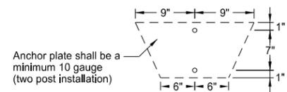
Anchor plate shall be a minimum 10 gauge (two post installation)
