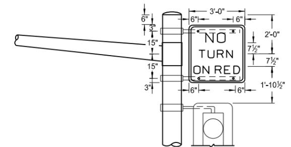
Signal Standard Mounted Sign Attachment Detail
