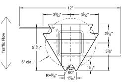
Bottom Soil Stub Tube - 3"x3"x7 gauge ASTM A500 grade B tube Stabilizing Wing - 7 gauge H.R.P.O. ASTM A1011 Plate - ASTM A572 grade 50
