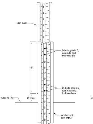
Breakaway U-Channel Splice Detail Alternate B (2.5 and 3 lb/ft)
