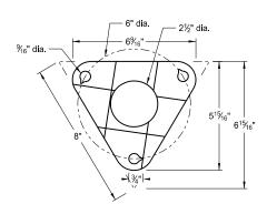
Bolt Retainer for Base Connection Bolt Retainer- 1/32" Reprocessed Teflon
