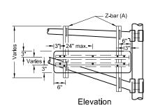
1/4"x2"x2"x2" alum. Z-bar or Sign to be centered 1/4"x2"x2" (2) alum. angle bars between top span wire and stability wire. - Bracket (see Detail A) U-bolt (C) - U-shape fitting 11/4"x3/8" dia. hex. head Perforated tube bolt, hex. nut, lock washer, metal washer, and nylon
