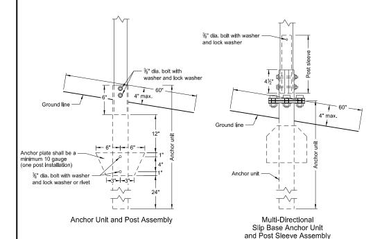
Anchor plate shall be a minimum 10 gauge (two post installation)
