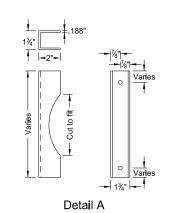
(A) Z-bar - Use  $1\frac{3}{4}$ " $x\frac{3}{16}$ " thick 1.08 lb/ft aluminum alloy. In place of Z-bar, two angles bolted together may be used or a channel.  $1\frac{3}{4}$ " $x1\frac{3}{4}$ " $x\frac{3}{16}$ " angles or  $1\frac{3}{4}$ "x2"x.188" channels.
