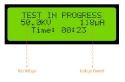
The VBT-75P S2 is Vanguard's second generation microprocessor-based, portable 75 kV dc vacuum bottle tester. This lightweight, portable tester is designed for testing circuit-breaker vacuum bottles in the field and at the shop.
