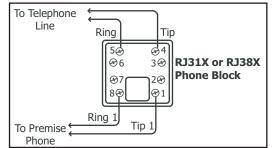
Figure 8: Phone Jack Wiring
