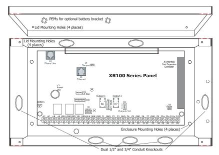
Figure 3: XR100 Series in Model 341 Enclosure
