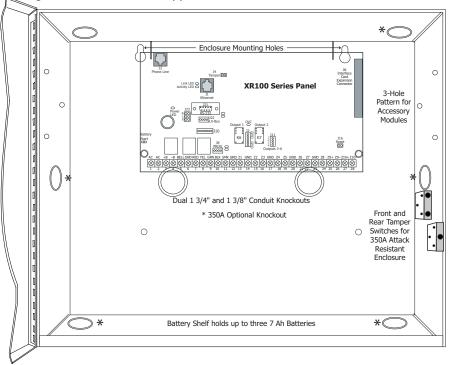
Figure 2: XR100 Series in Model 350 or 350A Enclosure
