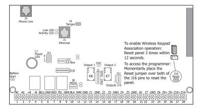
Figure 9: XR100 Series Panel Showing the Reset Jumper
