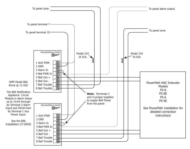
The Bell Output programming for Fire type zones must be set to Steady
