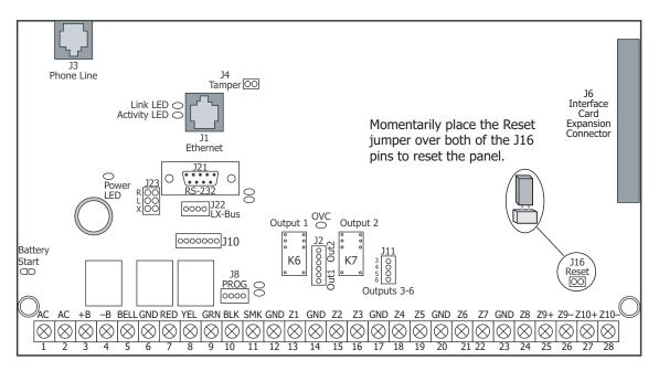
Figure 12: XR500 Series Panel Showing the Reset Jumper
