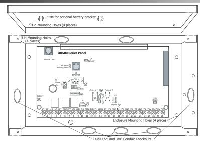
Figure 3: XR500 Series in Model 341 Enclosure
