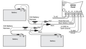
For listed installations, all batteries shall be installed
