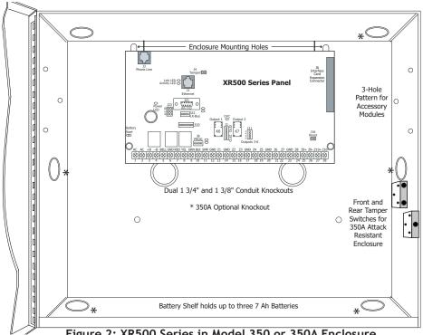
Figure 2: XR500 Series in Model 350 or 350A Enclosure
