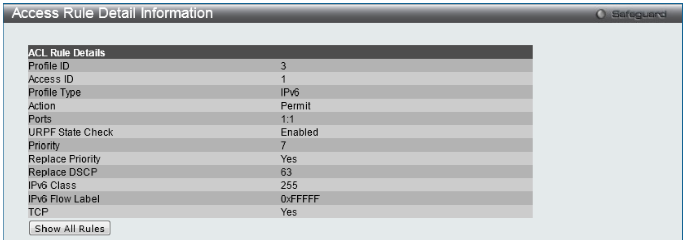
Figure 8-17 Access Rule Detail Information (IPv6 ACL) window
