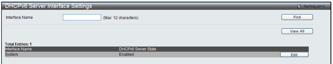
Figure 10-24 DHCPv6 Server Interface Settings window
