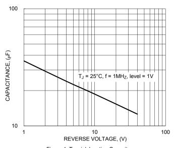
Figure 4. Typcial Junction Capacitance
