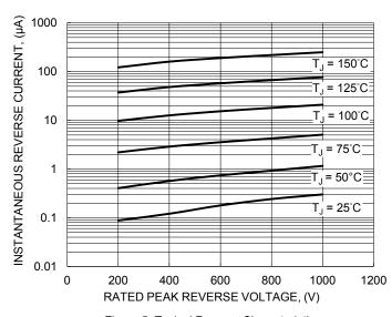
Figure 5. Typical Reverse Characteristics
