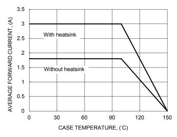
Figure 1. Forward Current Derating Curve
