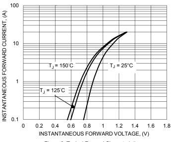
Figure 3. Typical Forward Characteristics
