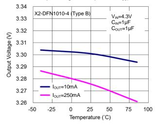
Line Regulation vs. Temperature, V<sub>OUT</sub>=3.3V
