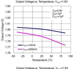
Output Voltage vs. Temperature, V<sub>OUT</sub>=1.8V
