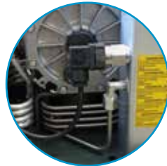
Pressure switch for automatic stop
