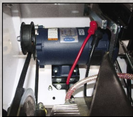
DC Travel option to allow movement of the saw when the saw is unplugged.
