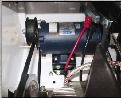
DC Travel option to allow movement of the saw when the saw is unplugged.
