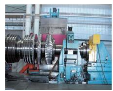
Indexing of the turbine shaft
