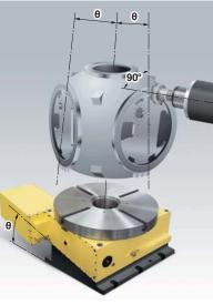
Configuration of the large rotary table on the horizontal M/C to machine a propeller hub of the windmill.
