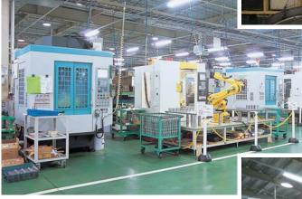
Small T/C and M/C line Utilizing small CNC rotary tables, NC5-46 toolings and Major Dream holders, this is highly sophisticated for high productivity line.
