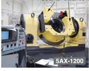
Testing of 5AX-1200 with counter balance weight
