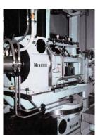
CNC400T is installed on CNC600V.
