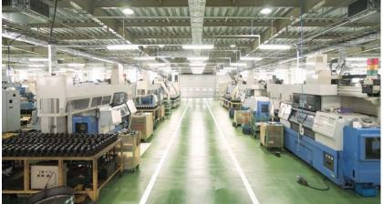
NC Lathe Lines Unmanned NC lathe lines are in full operation with utilizing of the Oil Jetter System and Combat Z Drills.
