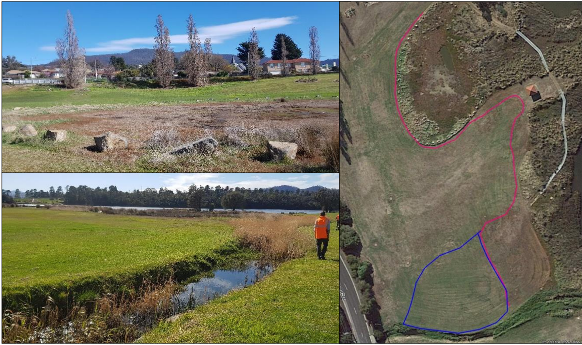
Figure 5-4. Windermere Bay. Top left: current saltmarsh area with boulders to be extended further. Bottom left: area alongside Faulkners Rivulet where marsh restoration work is planned. Right: red line indicates area for passive restoration by no-mowing; blue polygon indicates area for future active restoration by scalping topsoil. Images by DEP 3/9/2019.
