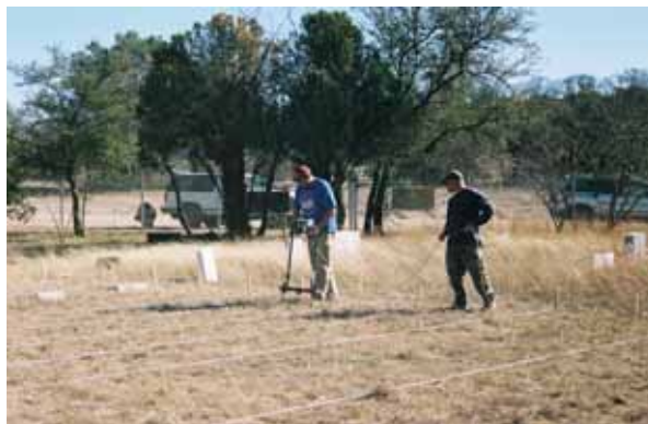
Figure 5.61. Resistance data collection at 0.50 m spacing, looking grid south. Note fence in farground of photograph.
