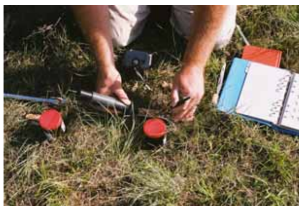
Figure 4.1. Photograph showing soil pH collection methodology for core samples.
