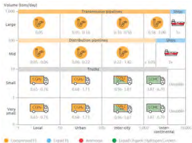
H 2 TRANSPORT COSTS BASED ON DISTANCE AND VOLUME, $/KG, 2019, (SOURCE: REPORT P. 60)
