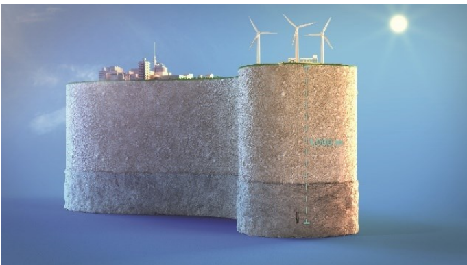
CONSTRUCTION OF THE HYDROGEN TEST CAVERN AT A DEPTH OF 1000 M (SOURCE: EWE GASSPEICHER GMBH)
