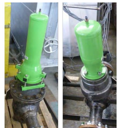
FIG. 3: UNIQUE MEASURING CELLS FOR EACH GATE VALVE (SOURCE: DBI)
