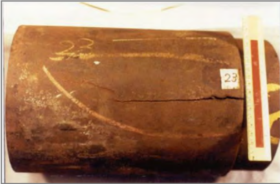
CRACK IN CASING BY HYDROGEN EMBRITTLEMENT (PETROLEUM RECOVERY RESEARCH CENTER, SOCORRO,NM)
