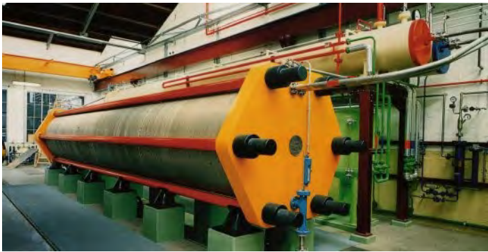
LEFT: IHT ELECTROLYSER TYPE S-556 (760 Nm 3 /h).
