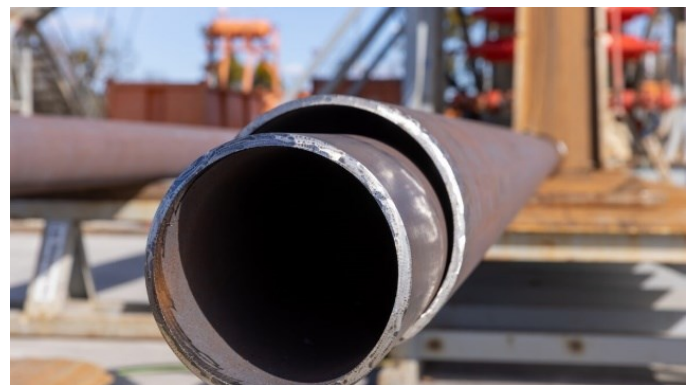
PIPE-IN-PIPE SYSTEM (SOURCE: ANDREAS PRINZ)
