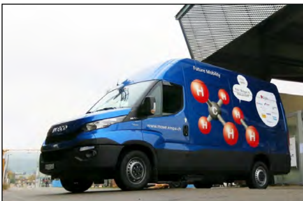
FIG. 3: PROJECT VEHICLE FOR HIGH H 2 -BLENDING RATIOS UP TO 30 VOL% (IVECO DAILY)
