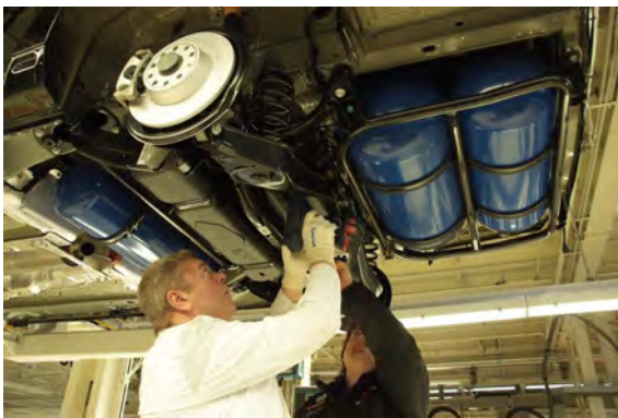
STEEL CNG1 TANKS (OZ-ONLINE)
