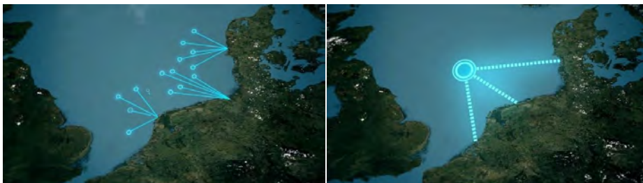
LEFT PICTURE: INDIVIDUAL NETWORK CONNECTION FOR OFFSHORE WIND FARMS RIGHT PICTURE: CENTRALISED CONNECTION VIA NORTH SEA POWER HUB (SOURCE: IMAGE FILM NSWPH)
