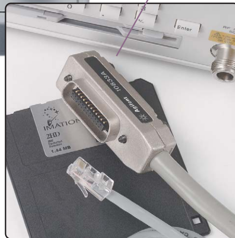
High-speed 10baseT LAN, parallel, and GPIB ports provide speed and flexibility when communicating with the outside world
