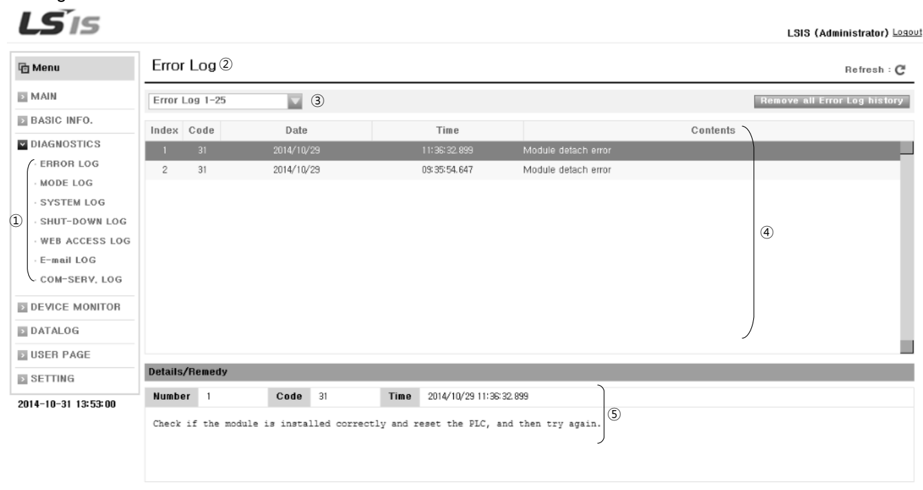
[Fig. 3.4.4.1] Composition of the diagnosis information (example of the Error Log)
