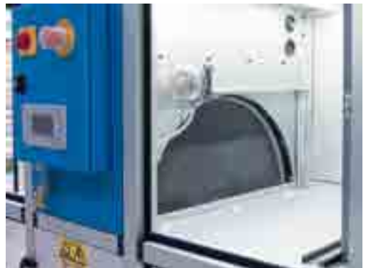
Heat wheel for heat recovery
