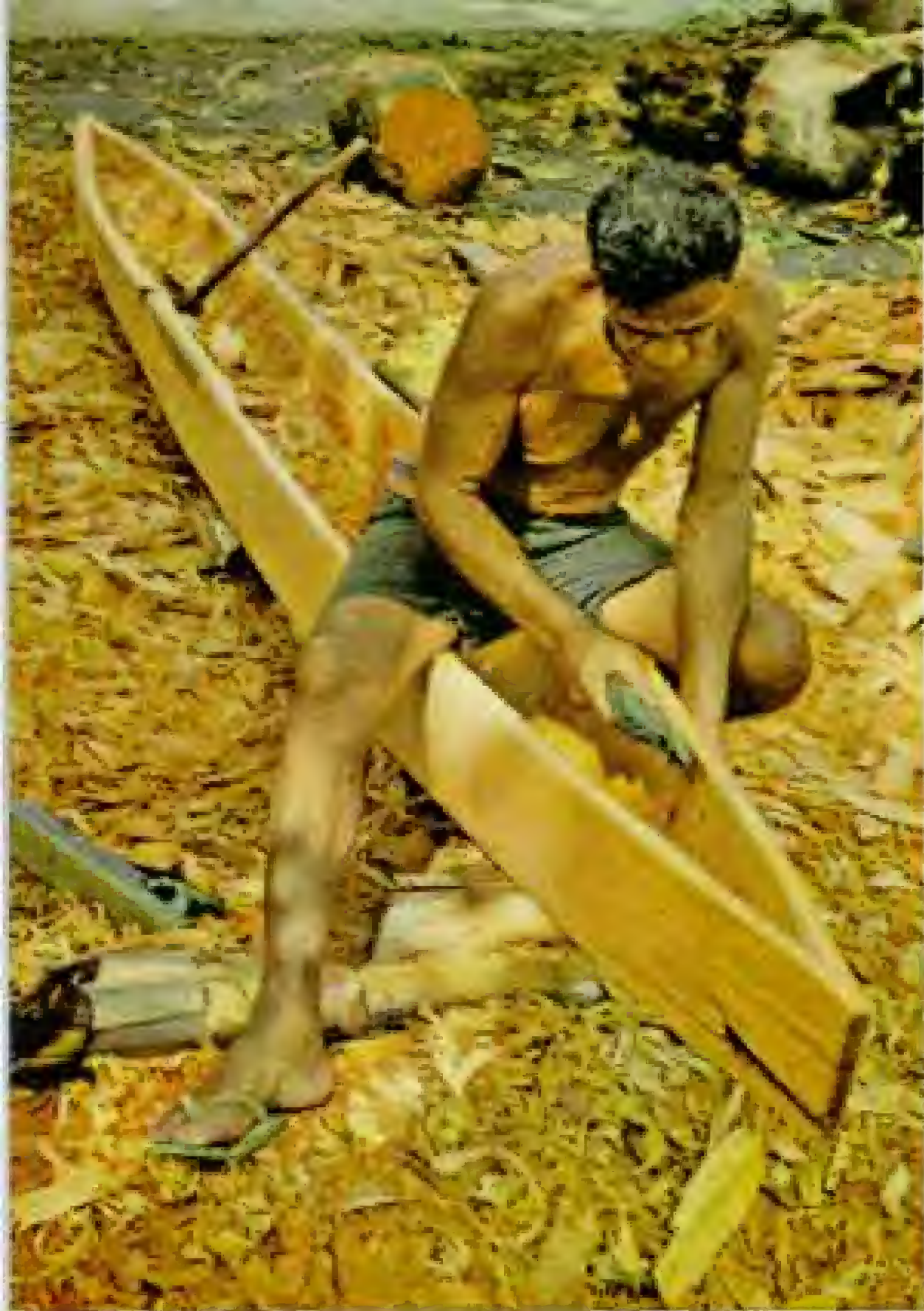
"Their Canoes . . . are built all of them very narrow," reported Captain Cook. With an adze, a master builder hollows out a log of breadfruit.
