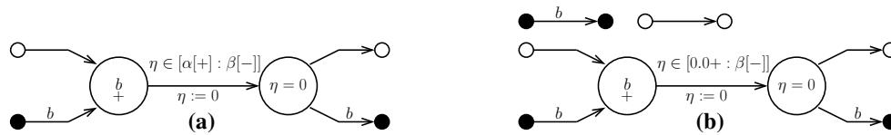
Fig. 4. Automata for (a) the Boolean smear, b[*\alpha[+] : \beta[-]] with a positive \alpha and (b) the Boolean smear, b[*0.0 : \beta[-]] with \alpha equal to zero.
